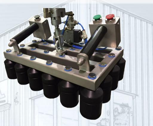
Prehension system for bottles, for the unpacking and packing of cartons and cases.
