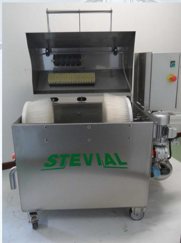
The washer has been made for the cleaning, by external brushing, of 20 to 50-liter beer barrels, without any adjustment. The cleaning rate depends on the time of the cycle that has been chosen.
